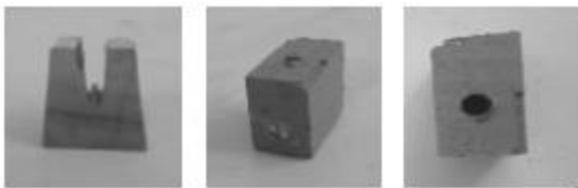
Fig 4:- (a) Groove making for hinged support, (b) Cube for joint connection (c) Drilling for joint connection
