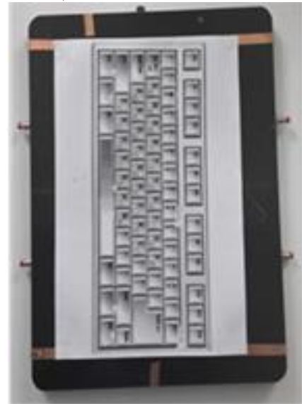
Fig 8:- The Capacitance Touch Panel As Computer Keyboard
