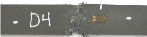
Fig 1:- Specimen after tensile test, from above
