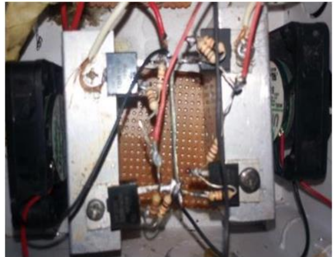
Fig 7:- Push Pull Circuit.
