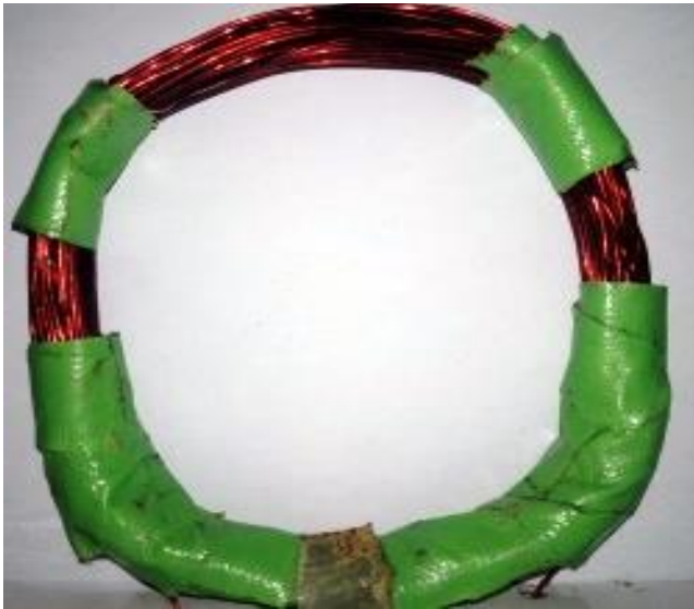
Fig 8:- Transmitter (TX) Coil
