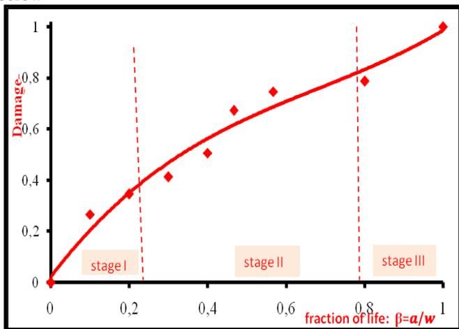
Fig 6:- Evolution of the damage as a function of the fraction of life for perforated and simply notched specimens
