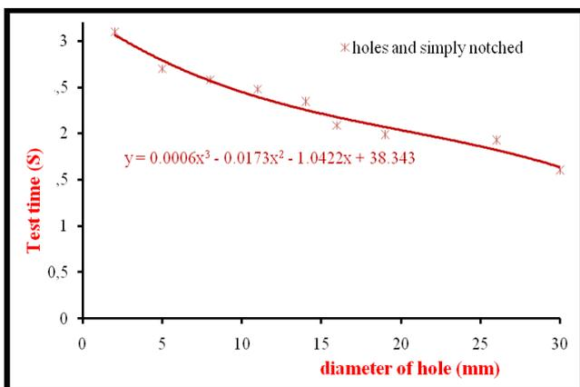
Fig 3:- The evolution of time of tensile test for perforated specimens and simply notched
