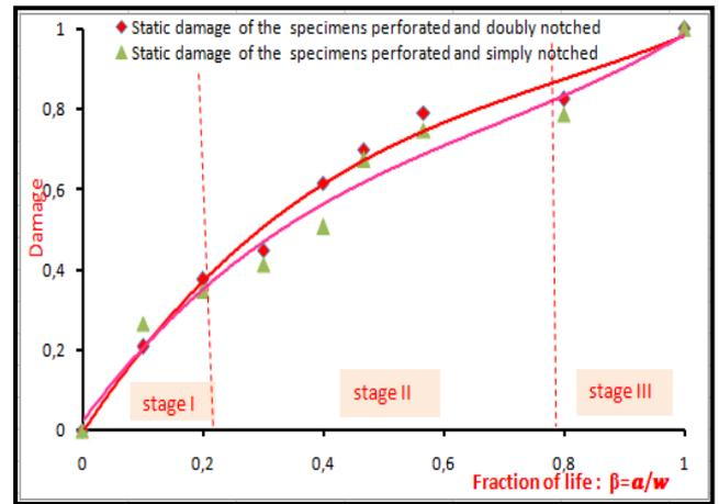
Fig 8:- Comparison between the damage evolution of the perforated specimen with single notch and the perforated specimen with double notch is according to the fraction of life.
