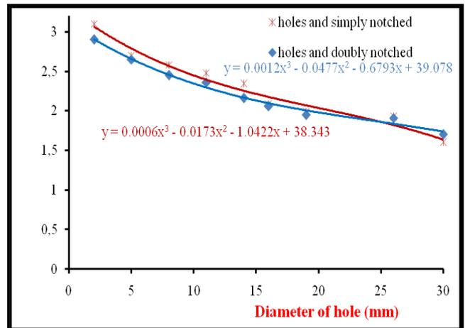
Fig 5:- Comparison of the evolution of test time between perforated specimens, simply notched and perforated test specimens, double notched according to the diameter of the hole
