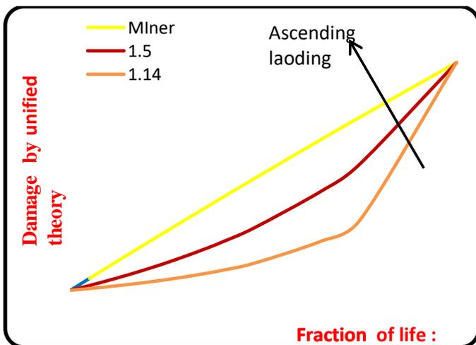
Fig 10. Evolution of Damage by unified theory and Miner law of the test specimens with double notch according to β.
