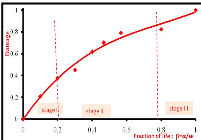
Fig 7:- Evolution of the damage as a function of the fraction of life for perforated and doubly notched specimens
