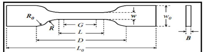
Fig 1:- Dimensions of the specimens according to ASTM D638-03 [4]
