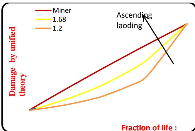
Fig 9. Evolution of Damage by unified theory and Miner law of the test specimens with simply notch according to the fraction of life.
