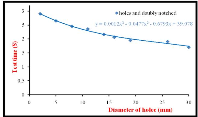
Fig 4:- The evolution of time of tensile test for perforated specimens and doubly notched
