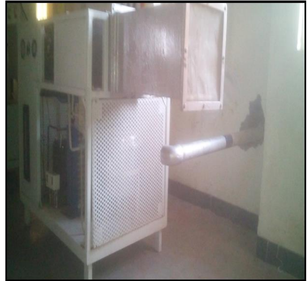
Fig 3:- EATHE Cold air supplied to Experimental setup
