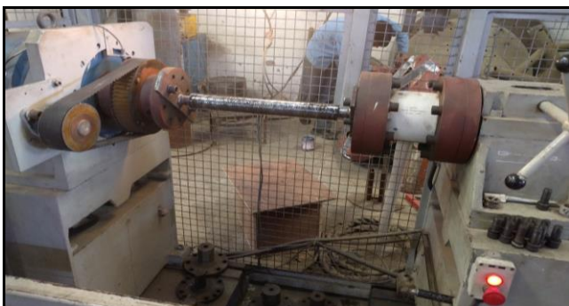
Fig 10:- Torque Testing of Composite Shaft
