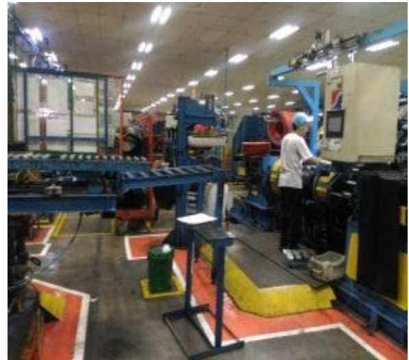
Fig 3:- Two Stage Building Machine
