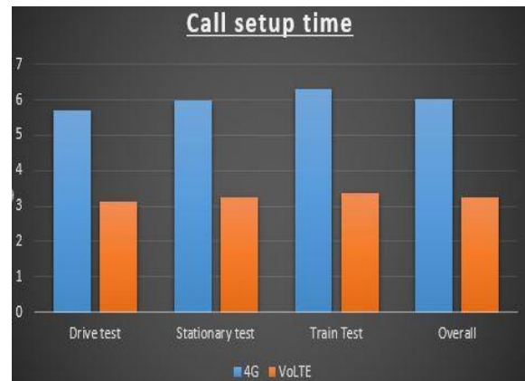
Fig 6:- Call setup time for mobility and stationary tests.
