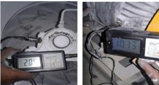
Fig 2:- The vibration data retrieval position
