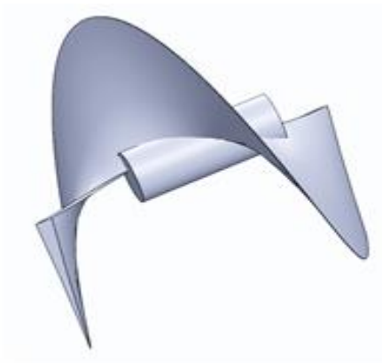
Fig 6:- Swept blade geometry
