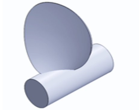
Fig 8:- Result of revolve cut
