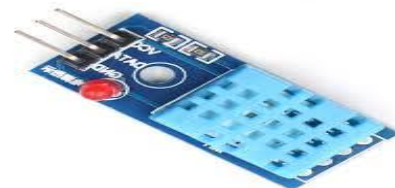
Fig 4:- Temperature & Humidity Sensor (DHT11)
