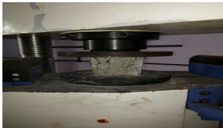
Fig 7:- Compressive strength test
