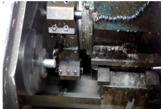
Fig 1:- Experimental setup for dry turning operation.
