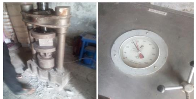
Fig 4:- Cubes Testing Process.
