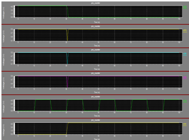
Fig 10:- Proposed Johnson Counter Waveform
