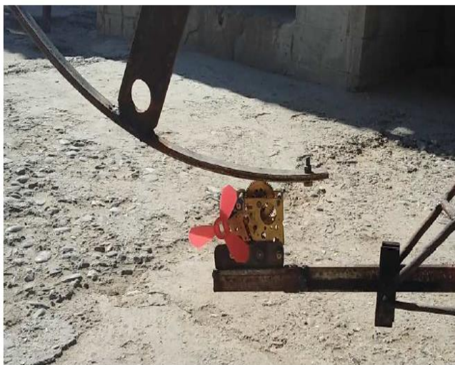
Fig. 4:- The small plastic propeller mounted to the output gear
