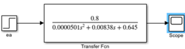
Fig 6:- Open-loop transfer function of DC motor without T_L
