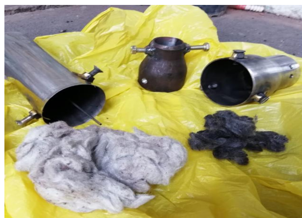
Fig 1:- Glass Wool Before and After Fixing to the Vehicle
