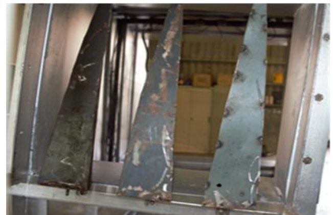
Fig 2:- Wedge-Turbulence Generating Mechanism
