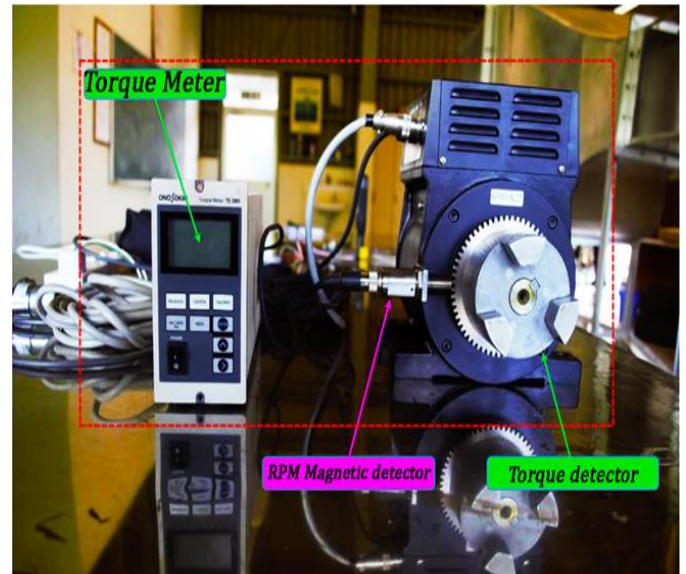
Fig 5:- Drive Side of the Torque Detector Model SS-500
