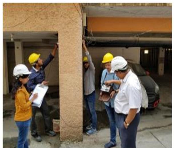
FIG 4: UPV Test by Direct Method for Column F3.
