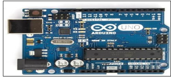
Fig. 1:- shows the Arduino board which acts as the microcontroller
