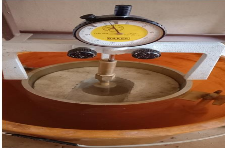
Fig 8:- showing Soil sample under soaked condition
