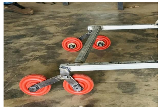
Fig 8:- Rocker arm system with wheels
