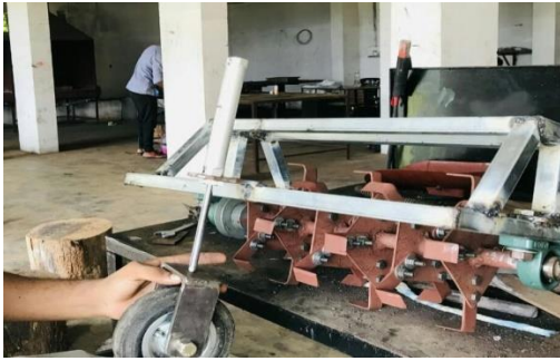
Fig 10:- hydraulic shock absorber coupled to the frame
