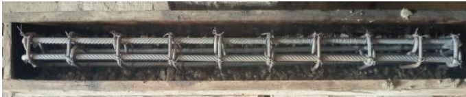
Fig 4:- Reinforcement inserted in mould during casting
