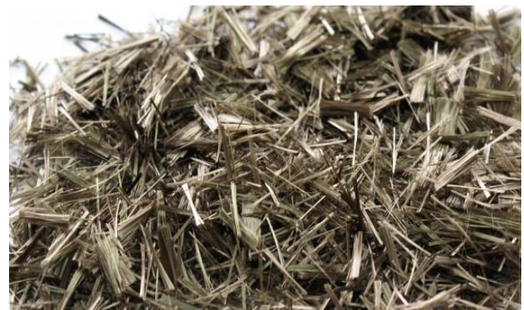
Fig 2:- Chopped basalt fibre (Borhan, 2013)
