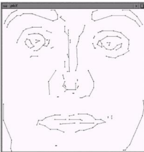
Fig 9:- Result of converting a face structure into line edge mapping [9]
