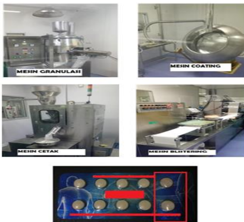
Fig 1:- Production Process of Solid Preparations
