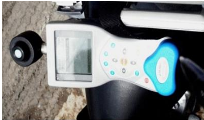
Fig. 2:- Measuring CO levels (CO Probe)
